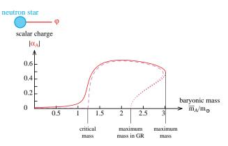
Figure 2: Dependence upon the baryonic mass  $\bar{m}_A$  of the coupling parameter  $\alpha_A$  in the theory  $T_1(\alpha_0, \beta_0)$  with  $\alpha_0 = -0.014$ ,  $\beta_0 = -6$ . Figure taken from [80].
