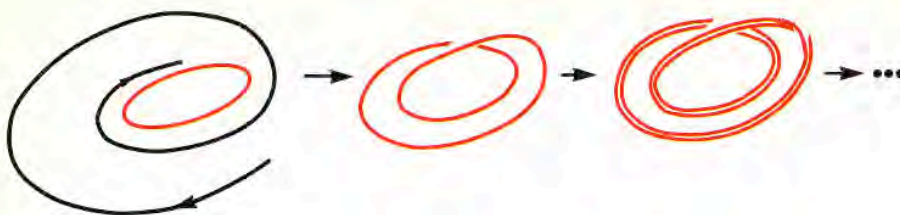
Bifurcation occurs when an attractor changes qualitatively in response to a small change in one of the system's parameters. In the example shown here, a limit cycle of period T is succeeded by a limit cycle with a period of approximately 2T (period doubling), which is in turn succeeded by one with a period of approximately 4T . The infinite repetition of this phenomenon is the Feigenbaum period-doubling cascade. Figure 3
