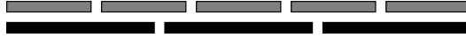
Figure 27: Vernier. Rodlike tiles differing in length form an assembly that grows until the ends exactly match.
